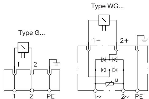
These connectors<sup>3)</sup> are part of the order coding as standard. For other connectors e.g. with clamp diode, economy circuit or LED's see D 7163.
