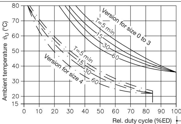
The curves do apply to stand-alone, individual valves only! If the valves are installed in a cabinet, it should be always equipped with louvers! In case of bank arrangement and ambient temperatures above 40°C the layout should be designed in such a way that adjoining solenoids are not energized over prolonged periods.
